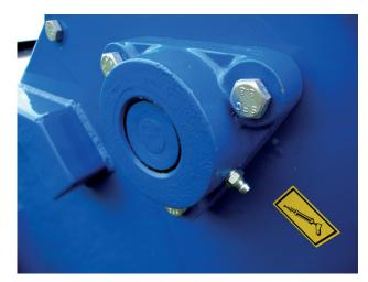
With slow moving shafts and no need for protective covers, bronze bushes which aren't affected by mud and silage have proven the obvious choice for our Bale Feeders. Proven over 30 years of use they are strong, simple and will give a longer life than bearings
