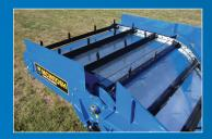
The trough feed arm extends to 2040mm from the centre of the tractor. A hydraulic ram raises the extension to help get through gates
