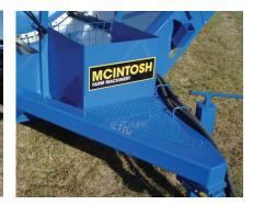
Checker plate to stand on when removing netting in one piece. The chassis goes through the cradle reducing the height. This greatly increases stability on hills
