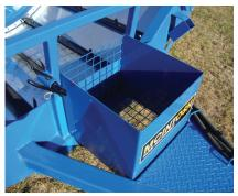
Steel box to hold plastic wrap. The mesh floor allows water and dirt to fall out and reduces the smell compared to an enclosed box
