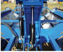
The double ram loading system lowers the bale gently all the way to the cradle without sudden drops which can damage feed out bars
