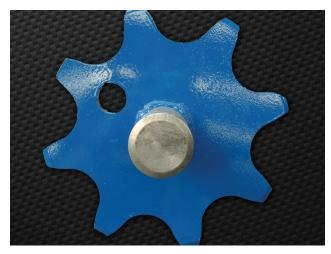
Large 8 tooth sprocket improves the life of the chain compared to a 6 tooth sprocket
