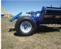
Standard tyres are 11.5x15.3, 50mm taller than the common 10.5x15.3 used on most double bale feeders. The taller tyre tows better over rougher ground than the smaller tyre
