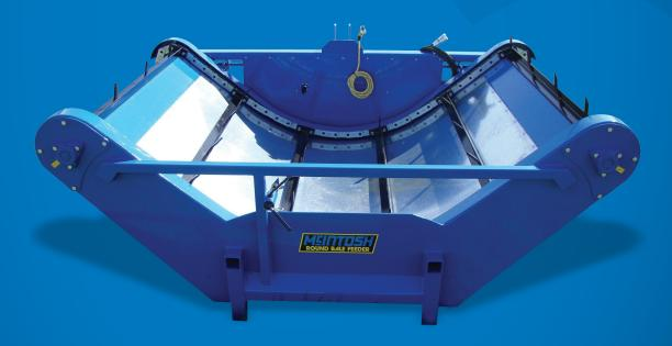
The cradle is intentionally short to help reduce the chance of bales twisting around and taking longer to feed out. The high front and back bars help stop the bale from falling out when travelling and feeding. A short cradle with end bars will feed out better than a long cradle with wasted room and extra weight out the back of the tractor. With no or short end bars bales can twist and fall out.
