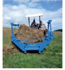
Optional fully adjustable square bale attachment with spring tynes. By being able to adjust both the tyne and angle of the bar, the attachment can be adjusted to suit
