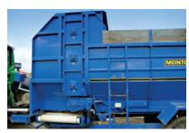
Side view showing beater attachment and hood, which channels feed onto the belt
