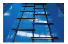
Floor chains: Three on the 800 - 1400 models Individual chain adjusters with a 40mm and two chains on the 500 - 700 models
