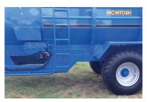
Stepped chassis to reduce overall height with the larger tyres on 1000 - 1700models
