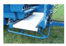
True bumper bars with extra brace on the corner to strengthen and protect the conveyor
