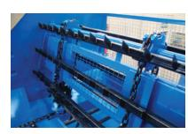
■ The elevator angle allows the front of the wagon to be fully loaded against, and will start every time without the need to back the load off
