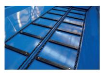
Optional four floor chains provide longer life for chains and sprockets
