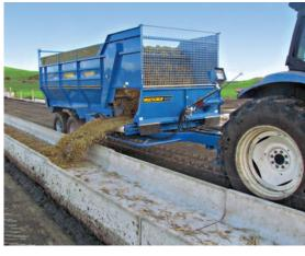
The long throw is ideal for feeding into troughs or under electric fences
