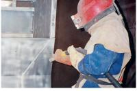
All machines are sandblasted and sealed prior to the application of our high quality paint system with a two-pack finish coat to give a durable lifelong finish
