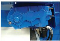
40:1 reduction gearbox for the floor drive eliminates the use of chains and sprockets, delivering more power direct to the floor
