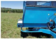
Cross conveyor slides out 200mm for trough feeding either manually (standard) or by the optional hydraulic ram
