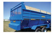
Heavy-duty back door made of 50 x 50 box section to help prevent bending
