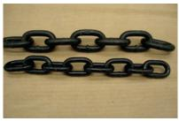
13mm floor and elevator chains used on the Titan Series, giving it double the strength of the 10mm used on Multicrop Wagons
